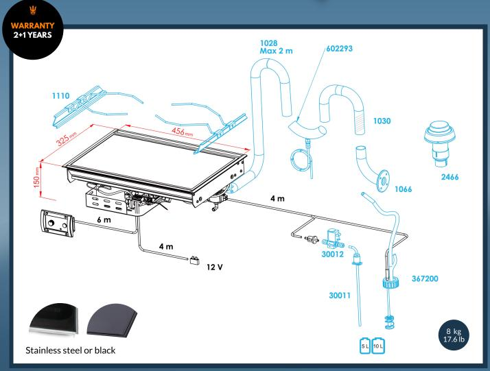
Accessories in black come with the standard package. Accessories in blue are additional. The calculated values are measured in a reference measurement wall, which is constructed to respond to a typical boat installation. The technical values have been measured with the maximum length of ducting, exhaust pipe, fuel line, and power cord. The figures allow for 10 % reserve - yours may vary.
