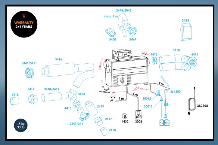
Accessories in black come with the standard package. Accessories in blue are additional. The calculated values are measured in a reference measurement wall, which is constructed to respond to a typical boat installation. The technical values have been measured with the maximum length of ducting, exhaust pipe, fuel line, and power cord. The figures allow for 10 % reserve - yours may vary.
