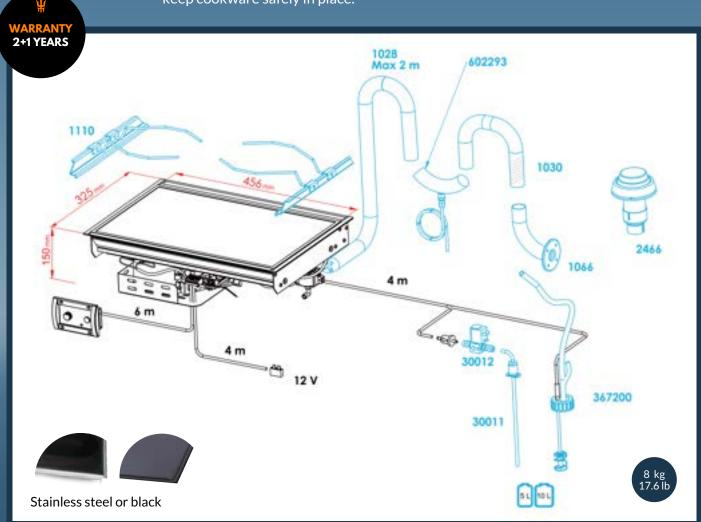
Accessories in black come with the standard package. Accessories in blue are additional/optional. The calculated values are measured in a reference measurement wall, which is constructed to represent a typical boat installation. The figures allow for  $10\,\%$  reserve - yours may vary.
