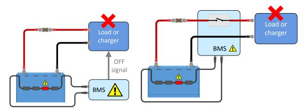
The BMS sends an on/off signal to a load or charger
