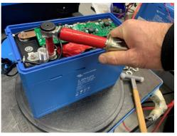
Loosen and remove the bolt that holds the positive circuit board wire cable lug.
