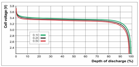
Discharge graph showing cell voltage at various depths of discharge for different discharge rates
