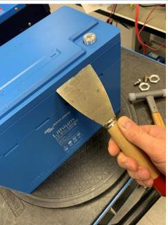
Carefully loosen or break open the lid. This can be done with a scraper, flat screwdriver or chisel.
