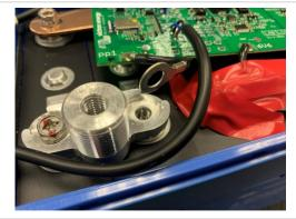
• Leave the positive circuit board cable lug disconnected for a few seconds.
