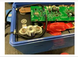
Insulate the negative busbar terminal located next to the positive battery terminal. Do this by covering the busbar with electrical tape. See red tape in the image on the left.
