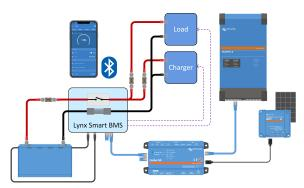
The Lynx Smart BMS will turn loads and chargers off via "load disconnect", and "charge disconnect" signals and controls the inverter/charger via a GX device. Should the battery be discharged even further, the BMS will disconnect the battery from the DC system.
