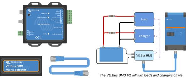
VE.Bus BMS V2, VE.Bus BMS Mains detector and RJ45 UTP cable
