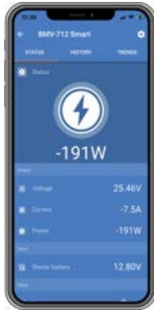
VictronConnect app status screen of a battery monitor running in DC monitor mode.
