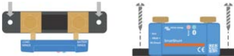
Top view SmartShunt IP65 indicating mounting holes and side view SmartShunt indicating mounting method.
