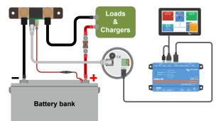
The battery monitor is connected to a Cerbo GX and a GX Touch screen.
