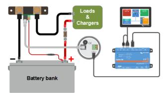
Example of a battery monitor connecting to a GX device.
