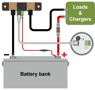
Basic battery monitor installation.
