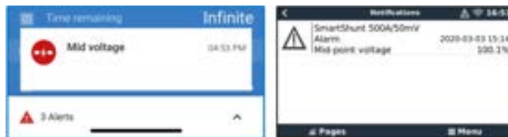
Left: alarm displayed on the VictronConnect app. Right: alarm displayed on a GX device.
