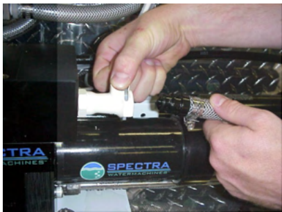
Connecting brine discharge service hose
