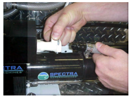
Connecting brine discharge service hose
