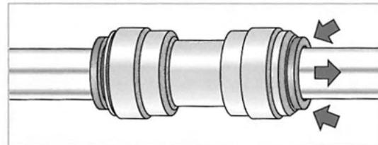
To disconnect, ensure the system is depressurized, push the collet square against the fitting. With the collet held in this position the tube can be removed.
