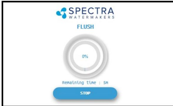
8. After Fresh Water Flushing the system will enter the 'Auto Store' mode, and the interval timer until the next scheduled flush will show on the screen.
