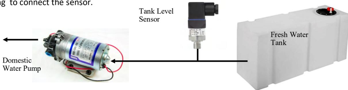
Route the 3 conductor cable back to the Spectra Connect control board at the feed pump module. Extend the wires as necessary. *If you must extend the wires beyond 50' contact the factory to ensure proper operation.*
