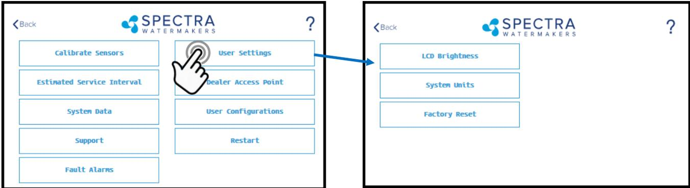
**LCD Brightness:** Set brightness of the hardwired display(s) from 10—100%
