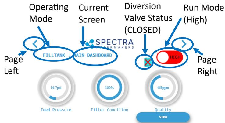
6. When the Product Water Quality is below the programmed threshold, the Diversion Valve opens, allowing water to enter the tanks and the screen image changes.
