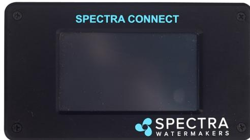
The Spectra Connect automatically monitors the operation of the system to ensure a long and trouble-free service life. If an operating parameter changes, the Connect can switch operating modes, shut itself down, or automatically store itself in order to protect your watermaker.
