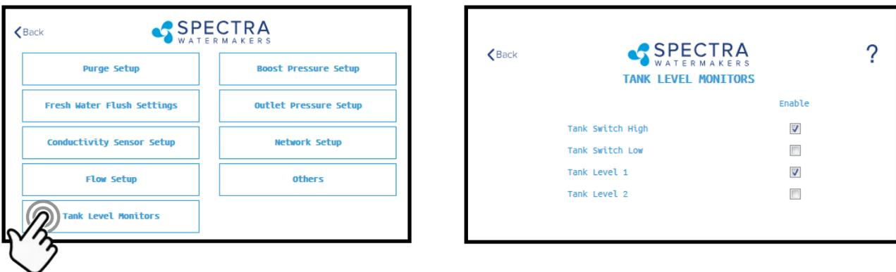
**Tank Setup** - Enable/disable tank sensors.
