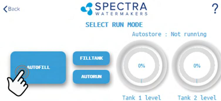
**WARNING: NEVER RUN YOUR WATERMAKER UNATTENDED. EQUIPMENT CAN BE SERIOUSLY DAMAGED, AND IT IS POSSIBLE TO SINK THE VESSEL!!** Use extreme caution when operating in Auto Fill mode!
