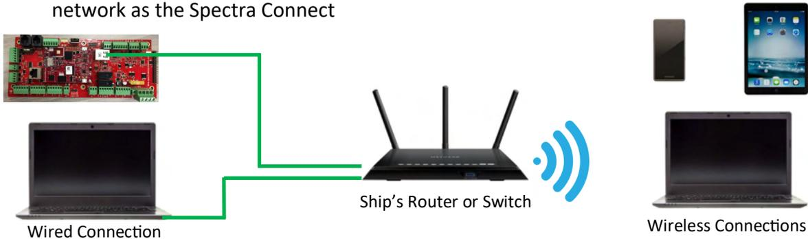
7. On the computer, tablet or smartphone, open a web browser such as Firefox, Chrome, or Safari. In the web address bar at the top, type the 'Device IP' address previously recorded. Press 'Enter'.
