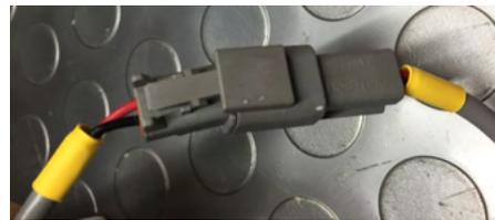
Connect the yellow boost pump connector from the Spectra Connect housing to the corresponding connector routed from the boost pump.
