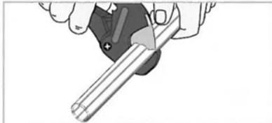
Cut the tube square and remove burrs and sharp edges. Ensure the outside diameter is free of score marks. For soft or thin walled tube we recommend the use of a tube insert
