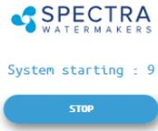
4. Once the Boost Pressure reaches the minimum threshold, the system starts operating and you will be taken directly to the Main Dashboard.
