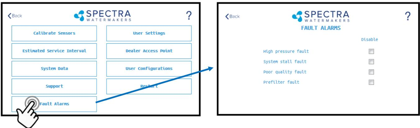
**CAUTION!!** Never disable a Fault Alarm without being certain that the issue is with a bad sensor. Disabling a fault and running the system can cause serious damage or injury.
