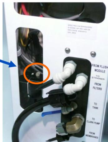
Push Diversion valve button down and turn 90 degrees to manually open valve
