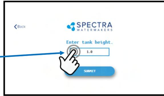
5. Measure the approximate height of the water tank in feet and inches (or in meters and cm's).
