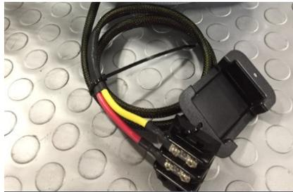
Mount the main power terminal block in a junction box or on a bulkhead adjacent to the feed pump module. Make sure that this is a dry location well above bilge level and not subject to water spray. **Be sure to install the terminal block cover.**
