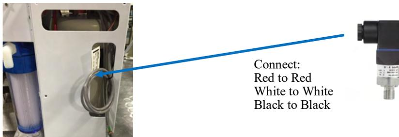
If a 2nd Tank Level Sensor is going to be installed, it should be installed at the base of the second tank. **If monitoring 2 water tanks, they must be isolated from each other with a valve to read properly.**
