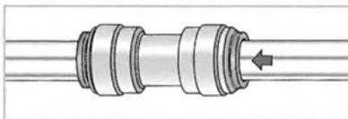
Push the tube into the fitting, to the tube stop.
