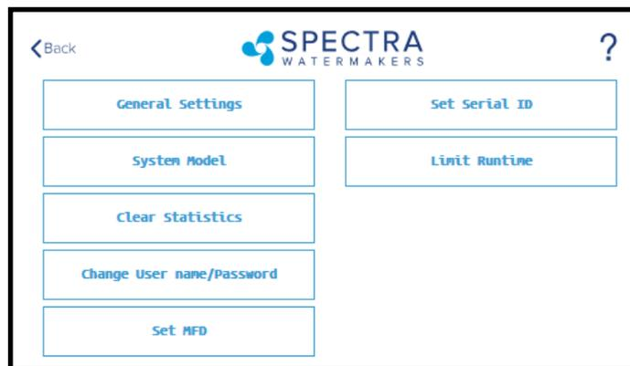
**System Model:** Configures the Spectra Connect for a different system model from a preset list of options.
