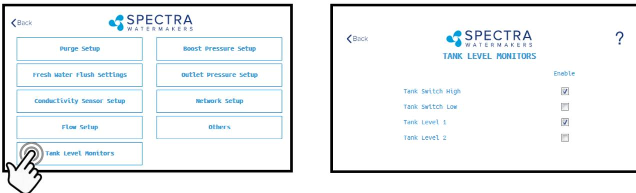
**Tank Setup** - Enable/disable tank sensors.
