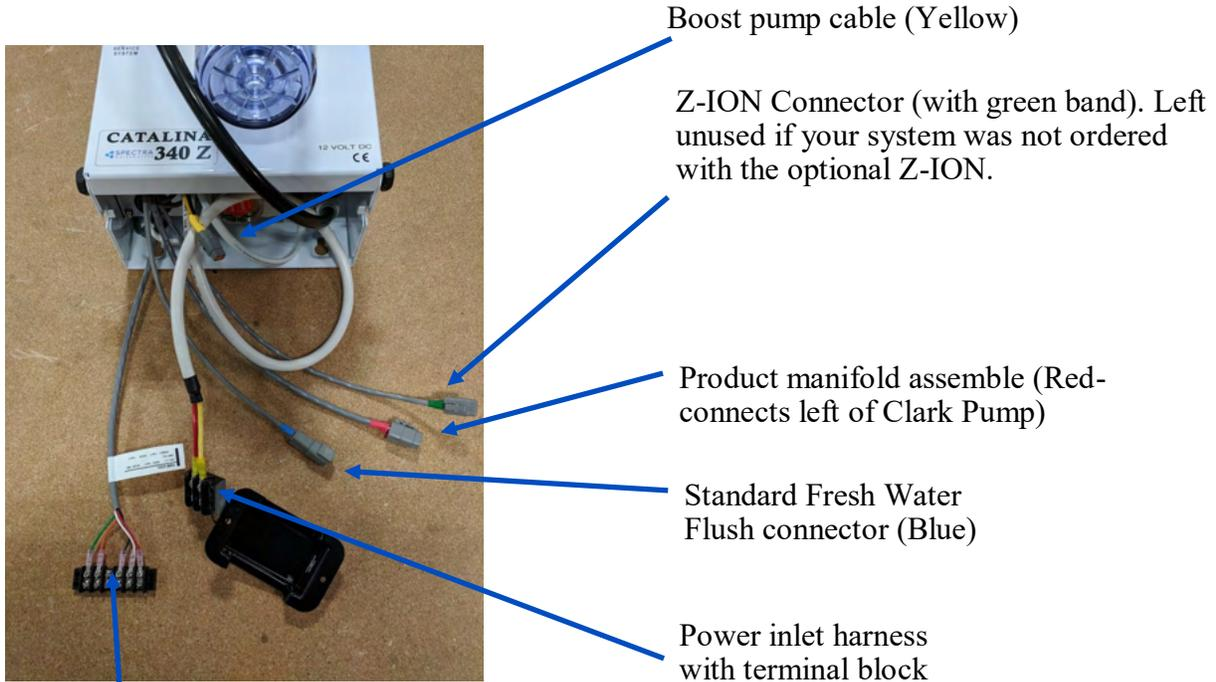
Tank Full Switch Terminal Block, Green + Orange
