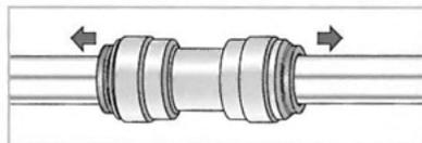
Pull on the tube to check it is secure. Test the system before use.
