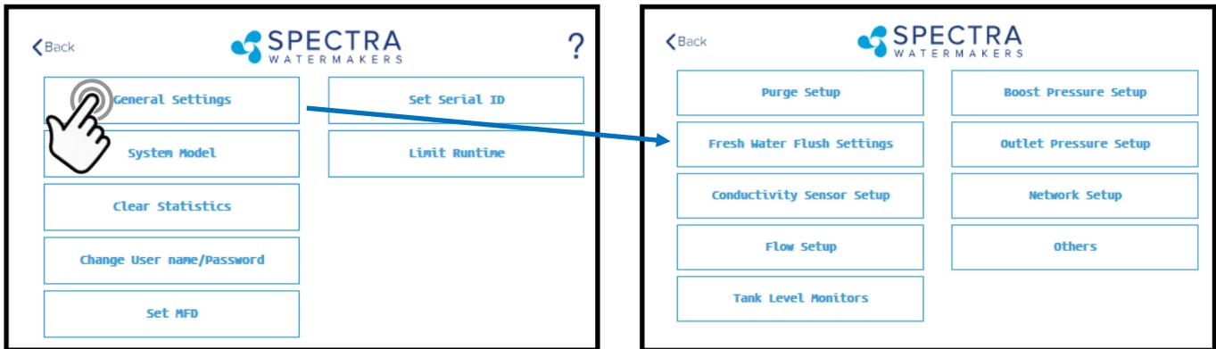
**Purge Setup:** Adjusts the time and maximum feed pressure allowed for the Purge Mode. **CAUTION: Permanent damage to the membrane can occur if this setting is adjusted. Consult the factory before making any adjustments.**
