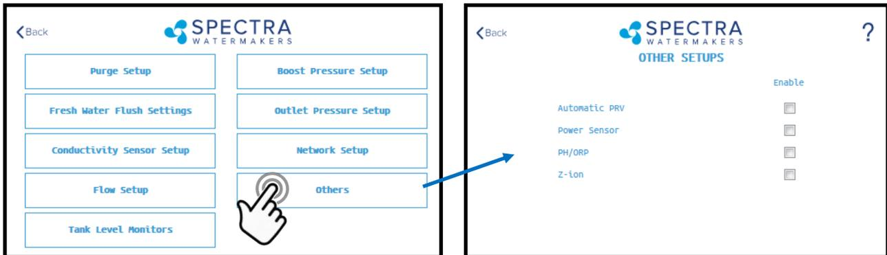
**Automatic PRV:** Enables an optional Automatic Pressure Relief Valve, after it is installed. This setting should remain off unless you are certain that you have this feature installed on your system.
