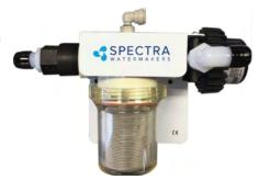
Fresh Water Flush Module: The fresh water flush module may be located in any convenient location near the feed pump module. It should be mounted with the filter housing vertical and accessible, with 2" below the housing for filter changes. Do not install over electrical equipment. The unit contains the charcoal filter, a solenoid shut off valve, and a flush water flow regulator.
