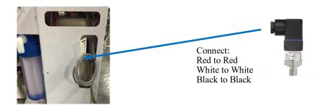
If a 2nd Tank Level Sensor is going to be installed, it should be installed at the base of the second tank. If monitoring 2 water tanks, they must be isolated from each other with a valve to read properly.
