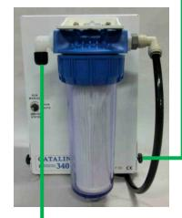
Use the supplied 3/4" (19mm) suction hose (clear with black spiral) from the inlet thru-hull to the boost pump/sea strainer module, and from the boost pump/sea strainer module to the feed pump.
