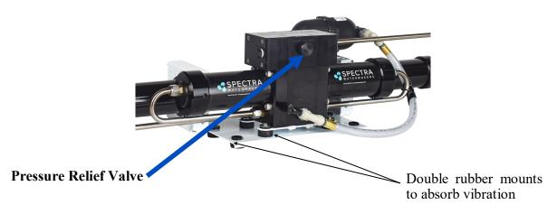
This module must be installed in an area that maintains a temperature below 113°F (45°C). It may be placed as high in the boat as you desire, and mounted in any position, even upside down. Make sure that the area around and under the pump does not have any water sensitive equipment, as water will be spilled during any repairs or if a leak occurs. Allow for easy access to the pressure relief valve.
