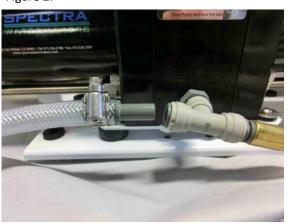
**Brine Discharge:** Route the brine discharge from the quick disconnect fittings to a thru-hull above the waterline using the supplied 5/8" braided vinyl hose and the male Quick Disconnect fitting from the installation kit:
