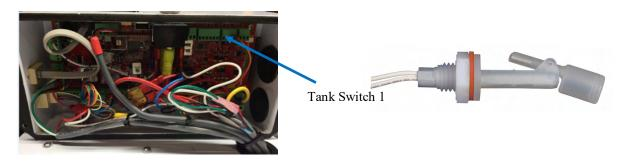
The float switch must be connected to the Tank Switch 1 terminals on the Spectra Connect control board at the Feed Pump Module. There is no polarity.
