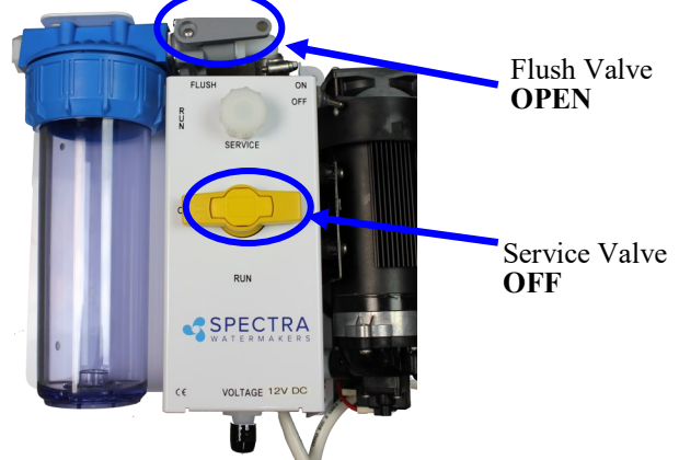
Feed pump module valves in FLUSH position:
