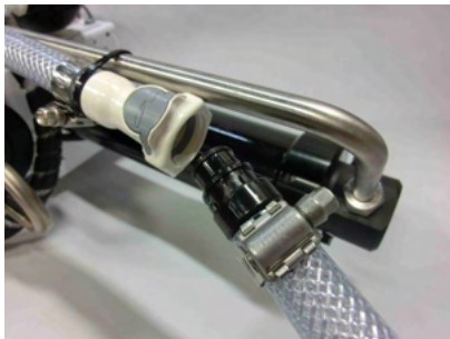
Connecting brine discharge service hose
