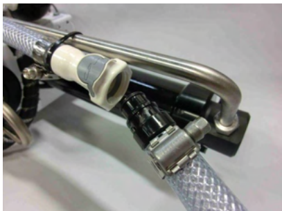
Connecting brine discharge service hose
