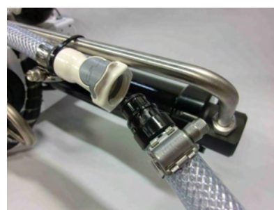
Connecting brine discharge service hose
