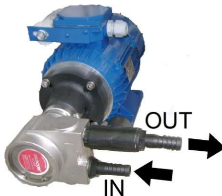
PUMP IN AND OUT FIG. 4-8
